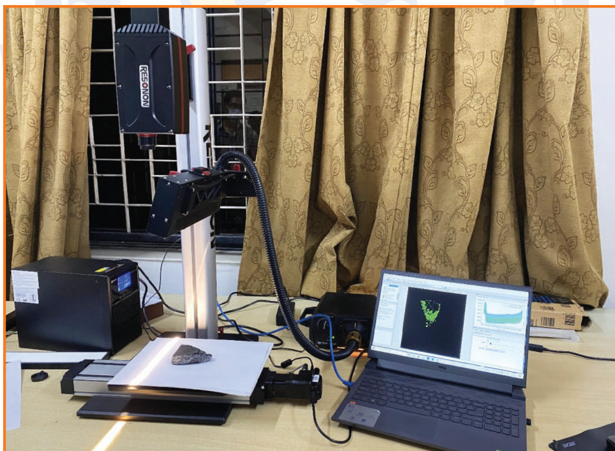
Hyper spectral imaging camera setup with light source and movable scanning
