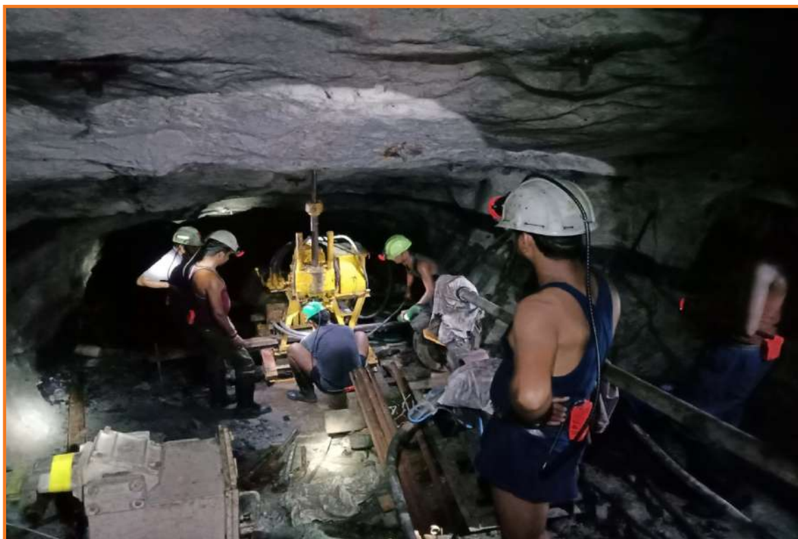
Underground drilling for coal gas desorption measurements for in-situ gas content determination
