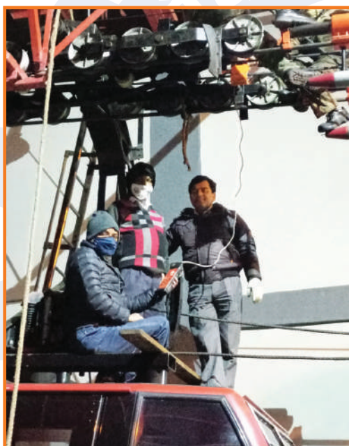
Non-Destructive Evaluation of Track Ropes and Haulage Ropes at Asia Resort Ltd. Timber Trail, Parwanoo, H.P.
