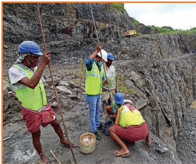
Fig.2: Conducting trial blasts and data collection at Cochin granite stone mine, Kerala
