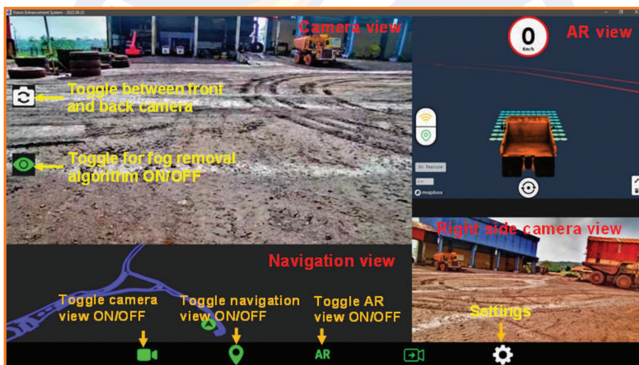
Fig. 4: Vision enhancement system's output display on touch screen PC fitted in front of the driver's seat
