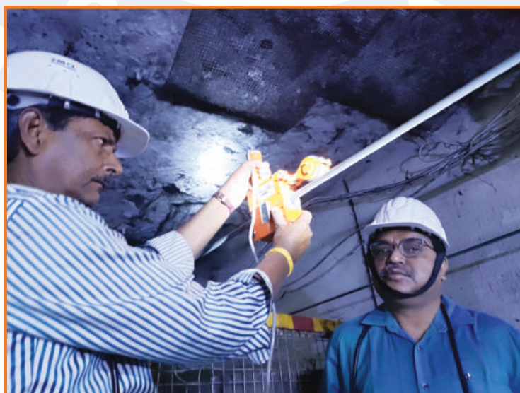
Evaluation of Haulage rope of Man Riding Chair lift at Nandira Colliery, MCL
